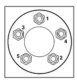
10. Tighten the wheel nuts firmly in a crisscross sequence as shown.
